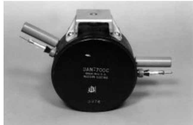
Fig. 9. Western Electric WE-700C magnetron, without its external magnet. Manufactured during World War II, it produced about 40-kW peak power at 690–700 MHz. Body diameter is 5.8 in (14.8 cm). Two of the output probes have protective covers installed (courtesy of the Historical Electronics Museum).
