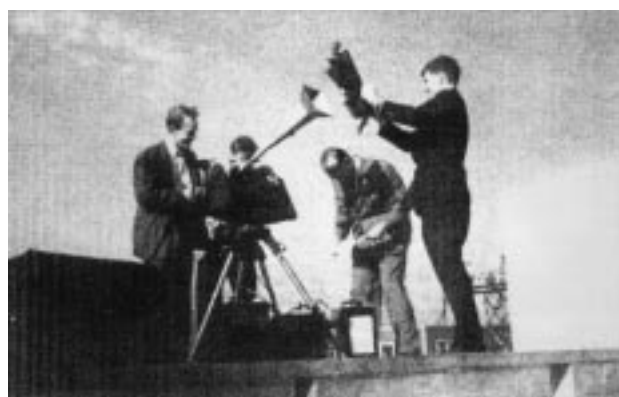
Fig. 11. Dicke (right-hand side) setting up a Microwave Radiometer to measure atmospheric thermal radiation at K -band (courtesy of MIT and [11]).
