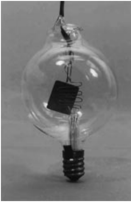
Fig. 4. Audion vacuum triode, 1908. Bulb diameter is 2 in (5 cm) (courtesy of the Historical Electronics Museum).
